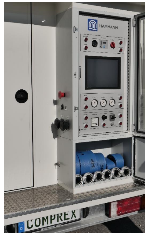
Figure 3: Touchscreen control and storage
